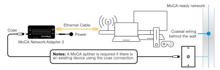
**IMPORTANT:** An existing MoCA-ready network or another ECB6250 Adapter is required. Internet availability should be delivered from your Internet service provider device (i.e., Cable or Fios modem/router).
