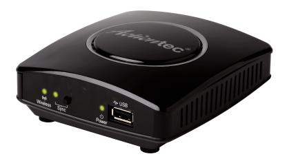
**Wireless LED** The Wireless LED, located on the front of the Receiver, is used to display the state of the Receiver's wireless signal. If unlit, the wireless radio is not on. If lit, the wireless radio is on.
