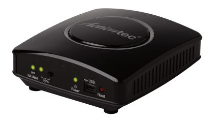
**Wireless LED** The Wireless LED, located on the front of the Transmitter, is used to display the state of the Transmitter's wireless signal. If unlit, the wireless radio is not on. If lit, the wireless radio is on.
