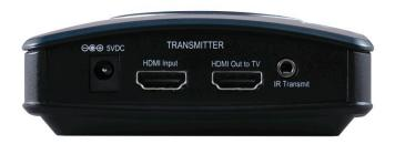
**Power Port** The Power port, located on the back of the Transmitter, is used to connect the Power cord to the Transmitter.
