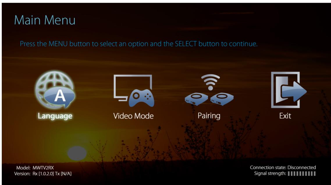
MyWirelessTV's Graphical User Interface provides system configuration abilities (Language, Video Mode, Pairing, and Exit) and displays system information (model name, version number, connection state, and signal strength).
