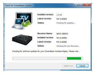
4. The Receiver's firmware update is performed first. Do not power off the Receiver during the update.
